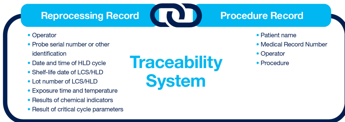
Figure 1. A traceability system links the information from the reprocessing cycle to the patient. The above information needs to be collected and linked to the patient for every HLD cycle. Adapted from AAMI ST58 and AORN Guidelines for periOperative practice. 1,2
