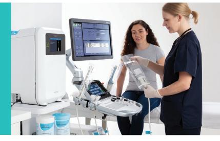
trophon is a state of the art point of care (POC) high level disinfection (HLD) device for ultrasound probes. The trophon family includes the trophon EPR and trophon2 devices, which share the same core technology of sonically-activated hydrogen peroxide.
