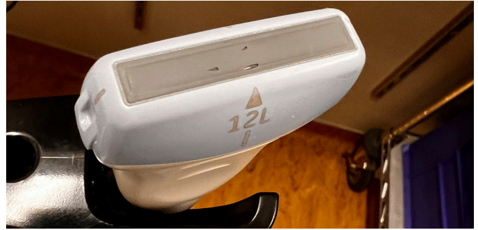
Figure 4. Gouge marks on ultrasound probes, indicating contact between the transducer head and needle during percutaneous procedures
